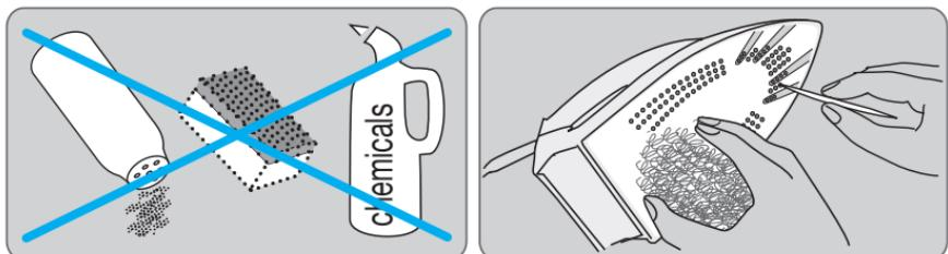
**G Cleaning the anti-calc valve**
